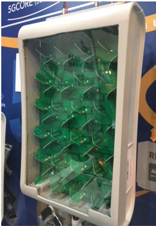
Figure 4: 5G ready base station with 44 cross-polarized antennas in a panel
