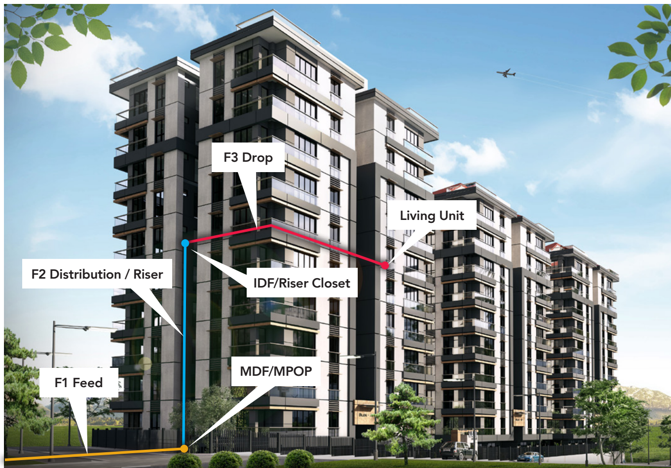
A Typical Cable Layout for MDU Fiber Deployment (F1/F2/F3 represent fiber cables)
