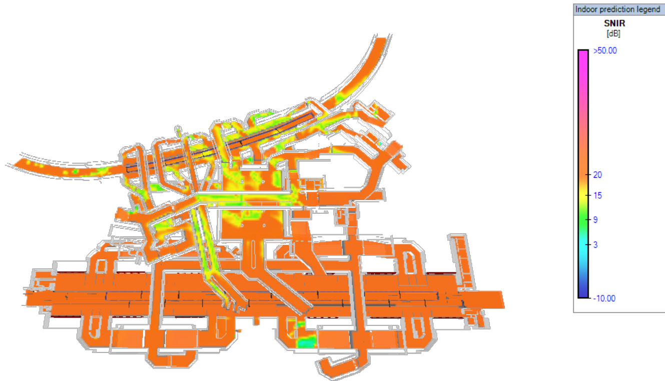
Figure 9: HSPA SINR Coverage used for Data Capacity Sizing Example
